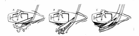
With an overtrimmed mainsail on a reach (A), the air flow breaks away from the leeward side of the sail. Similarly, with a closed leech (B), the air flow also breaks away from the leeward side of the sail. Both result in inefficiency compared with a correctly trimmed main (C) over which the air flow is smooth
